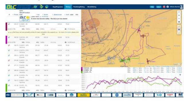
With the CTRL key and a mouse click, individual flights can be selected and displayed overlaid. It doesn't matter whether the flight is still being received in live mode or has already been claimed.
