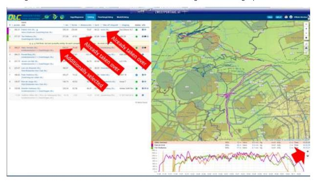
With the cursor in the barogram, they can now be analyzed well. A click on the small gear at the right side of the barogram also allows to synchronize the flights according to the start time. This can be very helpful for competition analysis.
